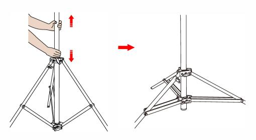
(1) If you want to get more stability, loosen the knob 1 & knob 2, the central column can be adjusted to a lower position but can't be below the legs, then lock the knobs tightly.
