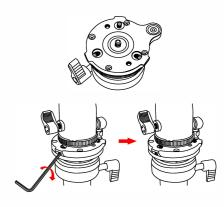
\*Notes: Three anti-twist screws prohibit unwanted rotation of tripod head, camera or other attached device.
