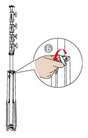
**2** Keep one leg against the ground, meanwhile hold the other two legs and spreader them (we recommend the open angle more than 30degree).
