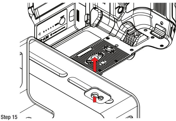
Slide the threaded studs into the channel of the base. Make sure they are aligned to the spacing of the holes on the riser plate.
