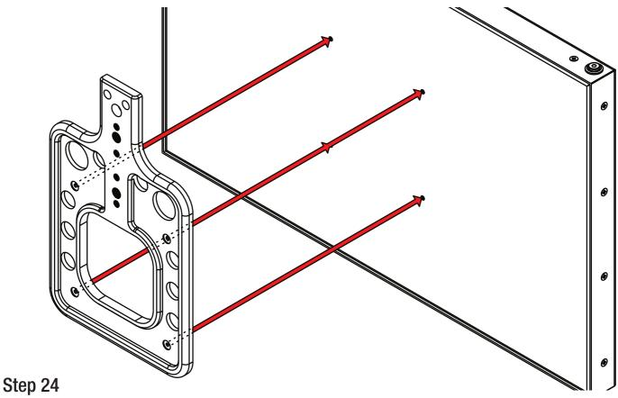
Attach the VESA adapter to the monitor by fastening the screws to the monitor
