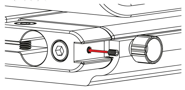
**Step 22**The headless screws should be inserted to the threads as pictured below.
