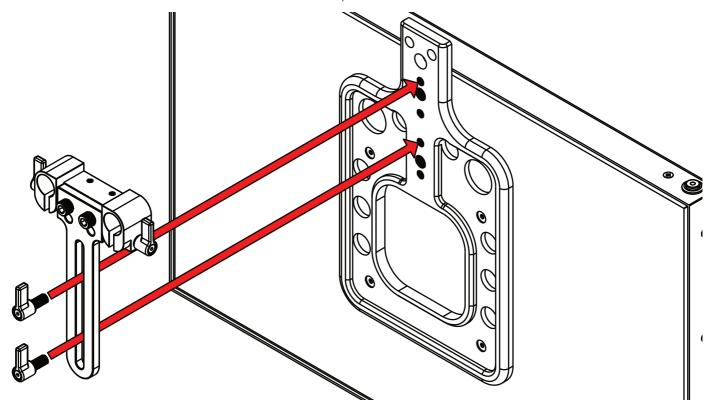
**Step 28**Fasten the screws to secure the Talent Monitor to the Rod Adapter.
