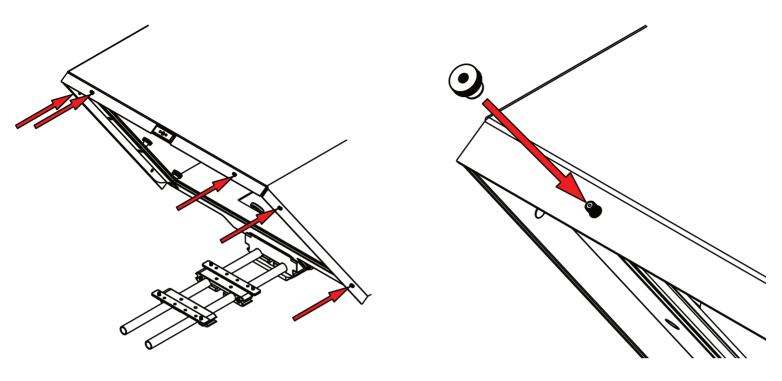
**Step 11**Fasten all six of the nuts to the threads on the hood frame to secure the hood to the teleprompter.
