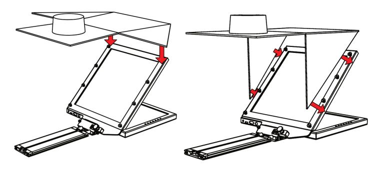
Step 9 To prevent light from leaking through the hood, seal both zippers down.
