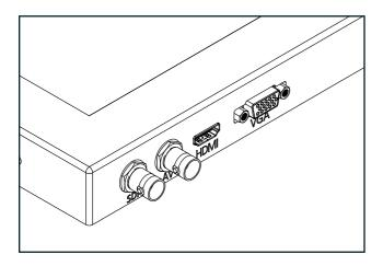
SDI – BNC Connection AV – Composite BNC Connection VGA – DE15 Connection
