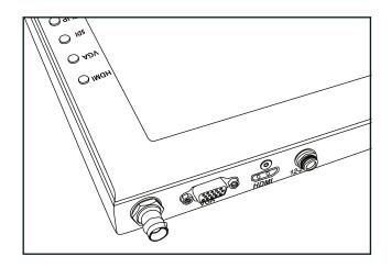
3G-SDI – Serial Digital Interface Connection VGA – Video Graphics Array DE15 Connection HDMI – High-Definition Multimedia Interface Input Connection Power Port – 12-24v Input
