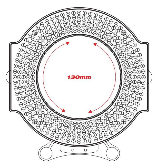
Insert screws through the 15mm/19mm Rod Mount and screw into the place on the ring light.
