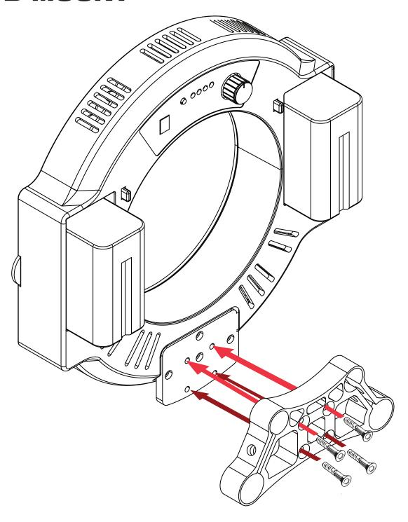
Insert Screws through the 15/19mm Rod Mount and Screw into the plate on the ring light
