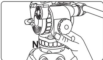
**9.2** To change the batteries, begin by reducing tilt drag and counterbalance to their lowest settings and make sure the tilt axis is unlocked. Tilt the head all the way back to expose the battery compartment, and lock the head in place with the compartment exposed.
