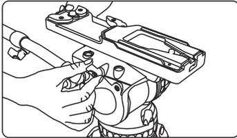
**4.3** Make sure the head's pan and tilt axis are locked, and attach the camera's VCT-14 wedge to the PS-C adapter. It will click when it is locked in place. Loosen the quick release plate lock and adjust the position of the camera to find the desired center of balance.
