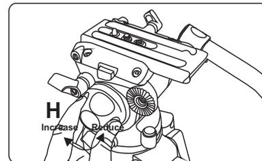
6. To mount a camera or camcorder, remove the quick release plate from the tripod head. Attach the plate to the camera using the included 1/4"-20 or 3/6"-16 screw. Take care not to over-tighten the screw.
