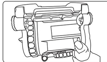
**10.2** If the battery must be changed, reduce tilt drag and counterbalance to their lowest settings and unlock the tilt axis. Tilt the head all the way back to expose the battery chamber, and lock the tilt axis.
