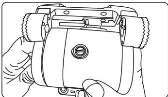
**9.3** Remove the battery compartment cover with a flat head screwdriver to access the battery chamber. The GH08, GH08L, GH10, and GH10L heads use 2x LR41 button batteries. Once the batteries are replaced screw on the battery cover and carefully release the tilt lock to return the head to its normal position.
