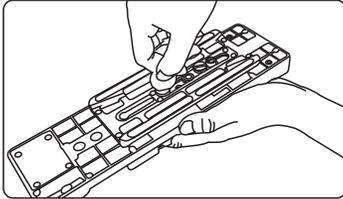
**4.2** Slide the quick release plate onto the tripod head. The plate release button will click when it is in place.
