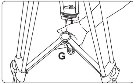
**b:** Holding the tripod by the bowl, lift up on the center of the mid-level spreader G and fold the legs together. Pull out the retractable easy hook D, wrap it around the legs, and secure the hook to a leg tube to secure the legs.
