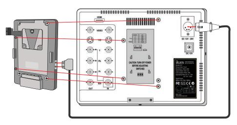
Install the M-A Battery Plate on to the VX7 monitor with the Phillips Head Screws.
