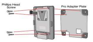
Remove the Phillips Head Screws to disassemble the M-A Battery Plate and the Pro Adapter Plate.
