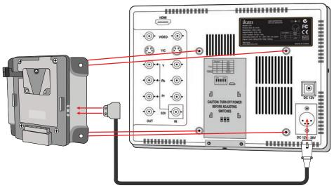
Attach the Pro Battery Plate to the VX9 monitor with four M4X.07 20mm Bolts.
