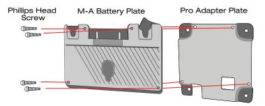
Remove the Phillips Head Screws to disassemble the M-A Battery Plate and the Pro Adapter Plate.
