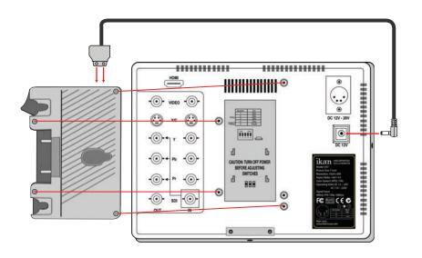
Install the M-A Battery Plate on to the VX7 monitor with the Phillips Head Screws.
