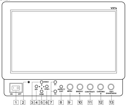
User programmable function buttons. For quick access, the user may program the F1 and F2 buttons to enable frequently accessed monitor features.
