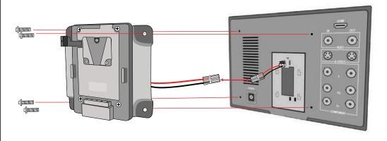
Connect both Pro Battery DC cables. Attach the Pro Battery Plate and the monitor with M4X.07 20mm Bolts.
