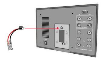
Insert the DC Cable in the connection slot.
