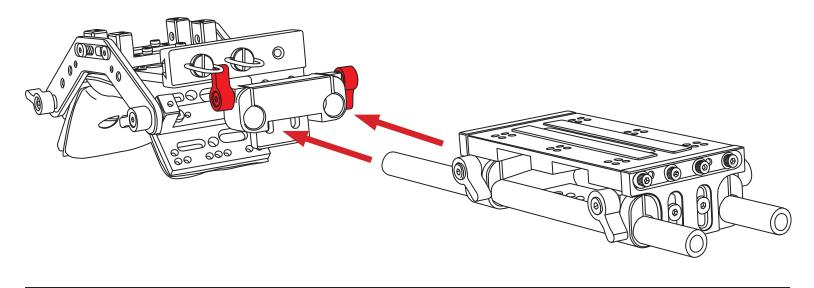
2. Next, connect the Grip to the Base Plate and tighten Thumb Screw [Ikan-TS].
