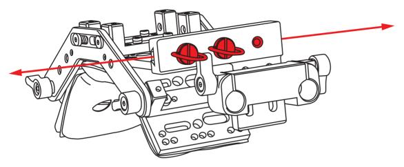
3. Vertical Adjustments to the Shoulder Piece can be made by loosening the Hex Screws located on the inside of the unit.
