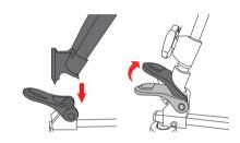
Attach the tripod or pedestal to the dolly. Please remove the camera from the tripod or pedestal before assemble the tripod to the dolly. Make sure that the leg bands at three positions are securely fixed.
