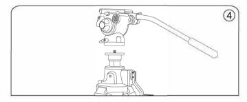
4. Fluid head or camera can be attached to the tripod directly.
