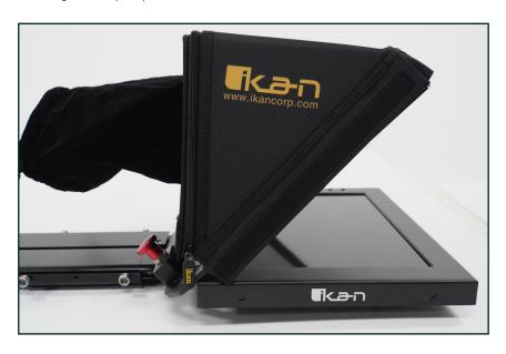
**Step 10**Slide the dual sided riser into the directional channel of the teleprompter base. Larger or taller cameras should insert the lower side facing glass, while smaller cameras should insert with higher side.
