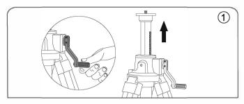
The geared center column will raise up when you revolve the crank clockwise, otherwise,it goes down.
