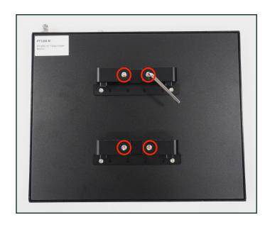
**Step 3**On the teleprompter base loosen the top 4 screws holding the rods in place.
