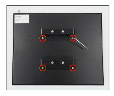
**Step 2**Using the larger hex key loosen the rod clamps.
