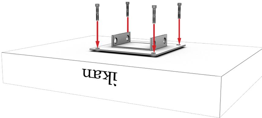
Then, attach four Phillips Head screws and four T-Slot nuts.
