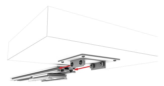
Attach four Phillips Head screws and four T-Slot nuts on the Prompter Glass Frame.
