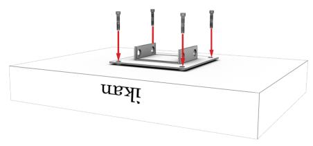
Then, attach four Phillips Head screws and four T-Slot nuts.
