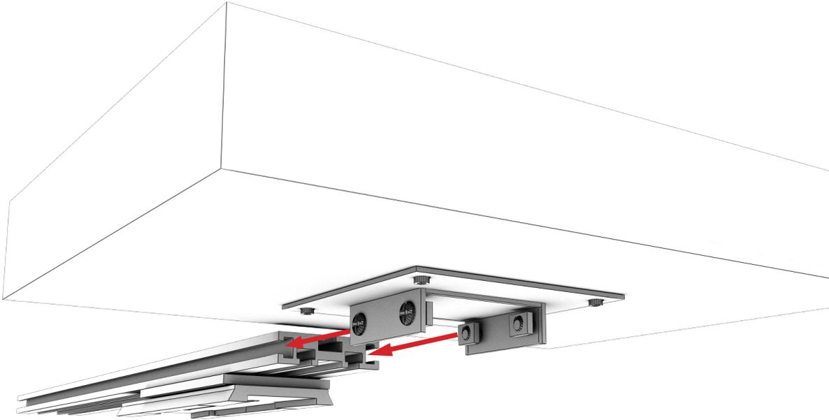
Attach four Phillips Head screws and four T-Slot nuts on the Prompter Glass Frame.
