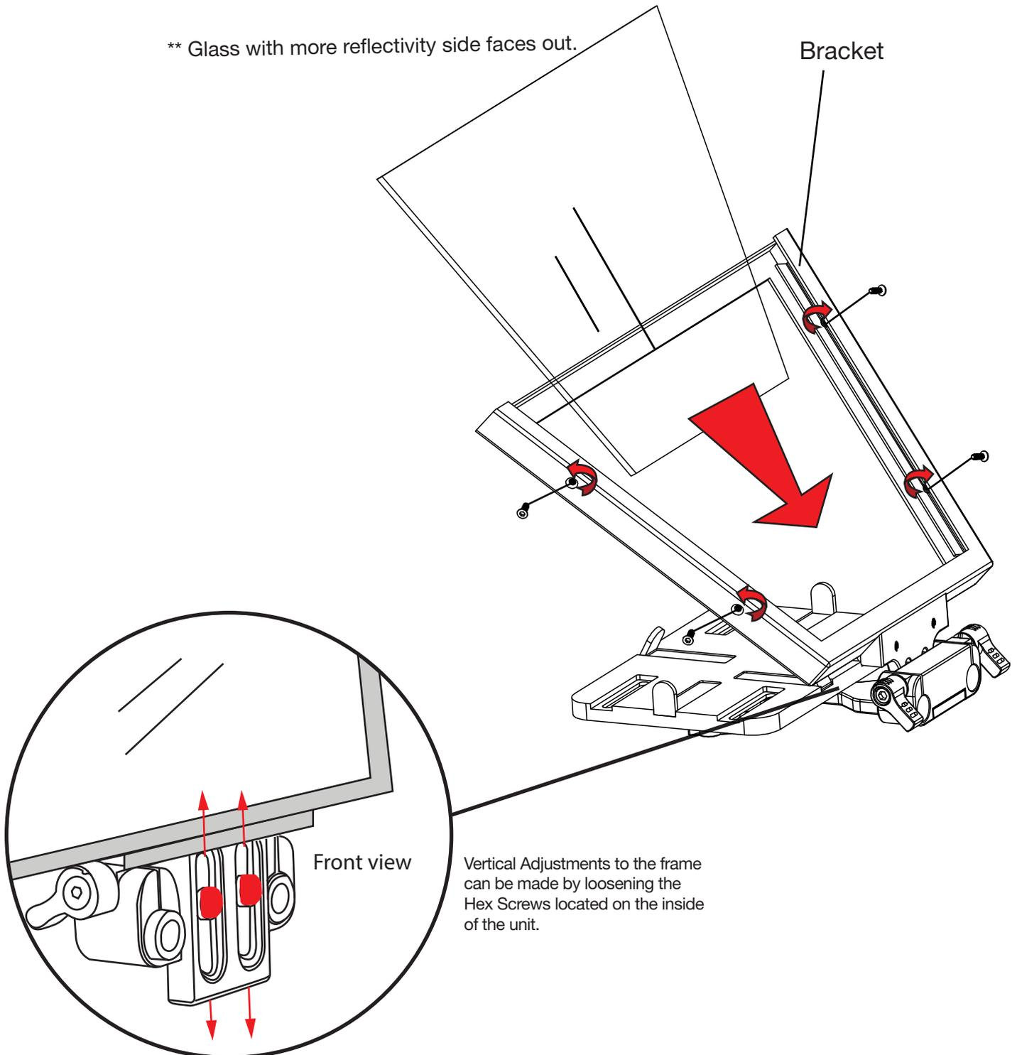
Vertical Adjustments to the frame can be made by loosening the Hex Screws located on the inside of the unit.
