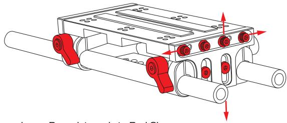
3. Secure Large Baseplate rods to Rod Clamp.
