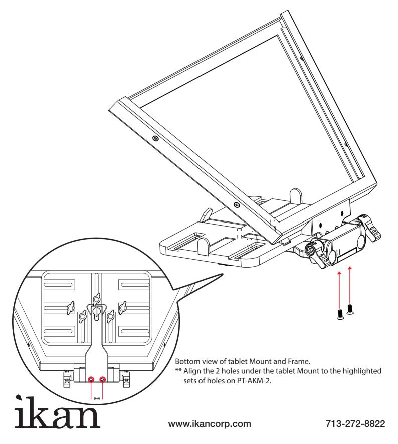
2. Remove 4 x small frame screws and 2 x brackets. Insert prompter glass into frame. Secure prompter glass by replacing brackets and screws.
