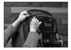
**Step 6:** Once the back flaps have been set take the two long elastic straps and attach them over the back of the light. (Note: Pushing the barn doors out from the front of the box through the diffusion will allow the box to stay on better.)
