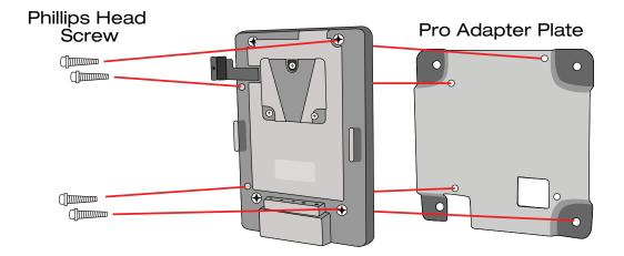
Attach the assembled plates to the monitor with M4x.07 x 8mm Metric Socket Head Screws. And, connect the Coax to Power Tap Cable.
