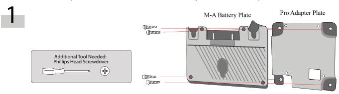
Install the M-A Battery Plate on to the VX7 monitor with the Phillips Head Screws.
