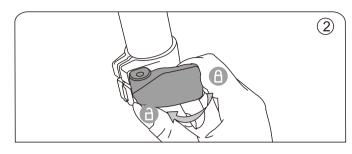
2. Open the flip locking to expand or collapse monopod tube.
