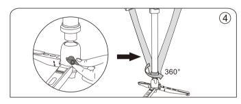
Loose the Wing locking knob, the monopod can swivel 360° and be tilted in any direction.
