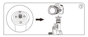
1. Camera can be attached to the monopod directly.
