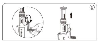
Geared center column provides extra height if you need to get your camera high up, it can be used on moving shooting and other events, which is easier to use than hand-head.
