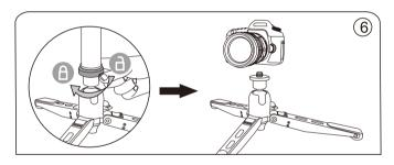
6.Loose the bottom base of monopod to remove the monopod, the mini leg can be acted as a mini tripod, make low angle shooting.
