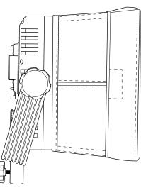
3. Once the outer frame is attached, the front diffusion panel can be placed on the light.
