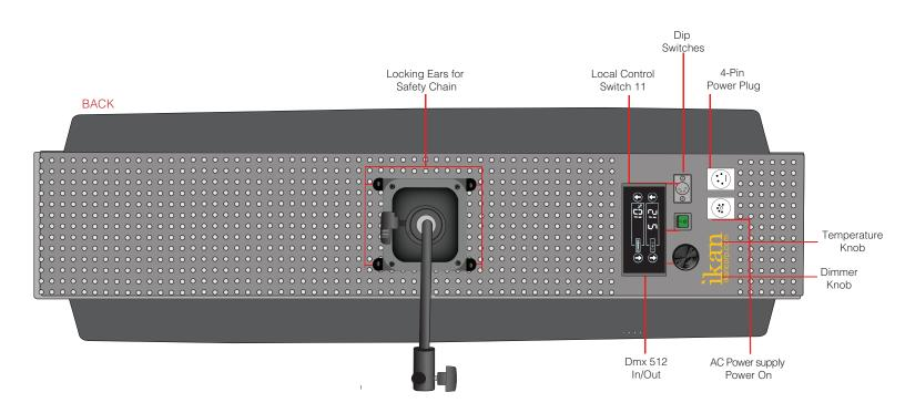
Attention: If not using DMX, make sure that DIP Switch #11 is in the ON position.
