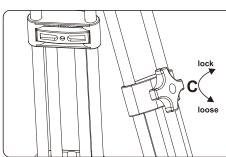
Important message: before unfold the tripod, please loose all the locking knobs "C", then adjust it to your requested length and lock it,
