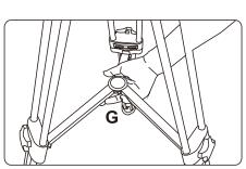
**b:** One hand catch the bowl base, another hand pull the middle spreader "G" and fold it. Then pull out retractable easy hook "D" and wrap around legs and bind them together.
