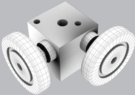
Gear box with wheels and riser
