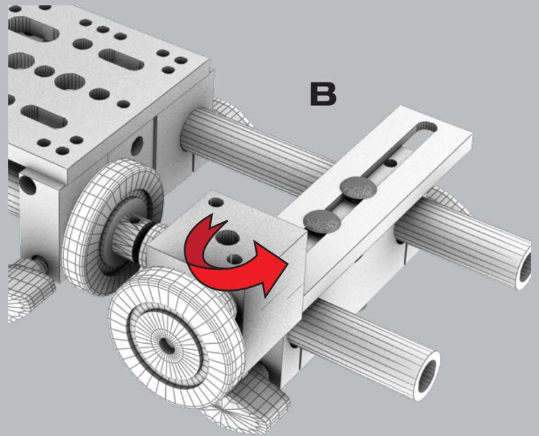
For shorter lenses, rotate the focus gear box to be closer to the camera body.
