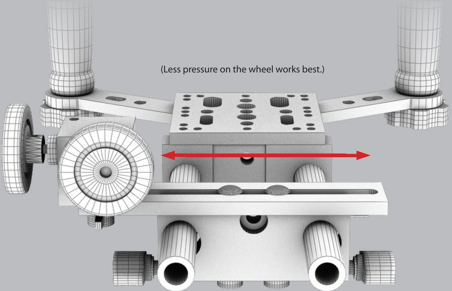
Gear box assembly can be adjusted as close to the lens as need be. The focus wheel should be snug enough against the lens focus ring that when turning the handle wheel, it will rotate the focus ring of the lens. The F3 is designed to work with most lightweight lenses. If the focus wheel fails to catch because the lens is too large in diameter or heavy, it is recommended that a geared focus option be utilized.
