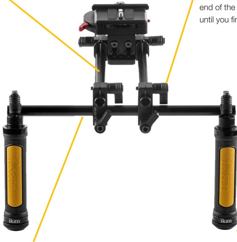
**3.** Slide the additional 12-Inch 15 mm rod through the bottom of the cross blocks. Once assembled, lock the cross blocks securely into place using the thumbscrews.
