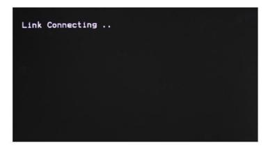
h) The system will spend 20-30 seconds on establishing the link, actual link period will depend on the current wireless channel condition. When the wireless link is set up the "RSSI" light will light up and indicate current wireless signal strength. The "Video" indicators will also illuminate and then the connected HD monitor will display the video and audio accordingly.
