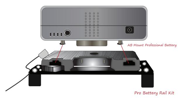
Loosen the thumbscrews to the Quick Rod Adapter and attach it on to your 15mm rail system and then tighten the thumbscrews. You can either mount that battery kit facing over or under the 15mm rails. To detach the quick snap battery kit, loosen the thumbscrews enough for the grips to clear the 15mm rails.
