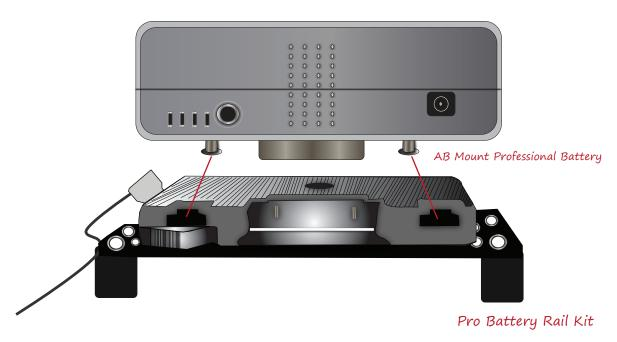
Loosen the thumbscrew to the Quick Rod Release Clamp and attach it on to your 15mm rail system for your BlackMagic Cinema Camera and then tighten the thumbscrew. You can either mount that battery kit facing over or under the 15mm rails. To detach the quick snap battery kit, loosen the thumbscrews enough for the grips to clear the 15mm rails and gently pull up.
