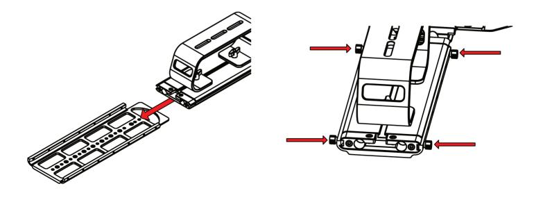
Step 15 To secure your teleprompter system, insert the included headless screws into the threads behind and in front of the Base.
