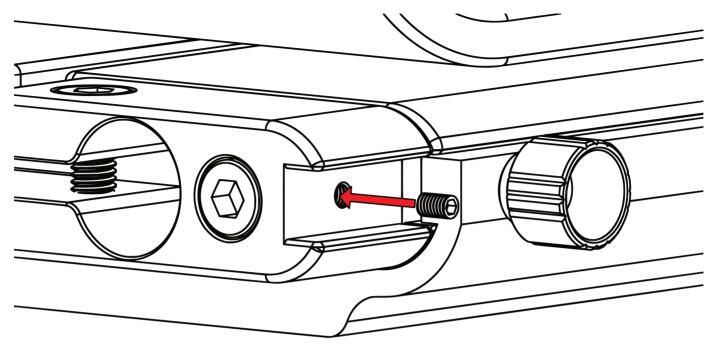
Step 16 The headless screws should be inserted to the threads as pictured below.
