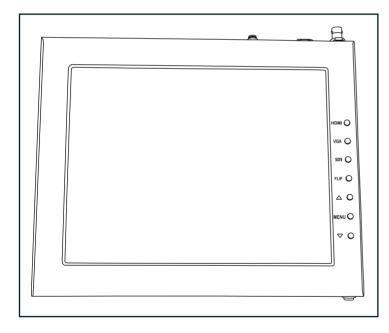
HDMI – Switch HDMI input VGA – Switch to VGA input
