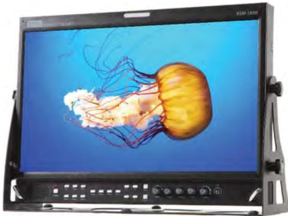
Being lighter and smaller in volume than a general 17" broadcast monitor, BSM-183H is an 18.5" super bright monitor suitable for outdoor shooting. BSM-213H is available for a larger full HD display (21.5")
