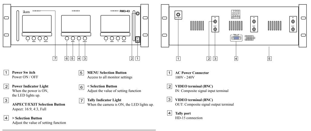
• For LCD panel adjustment sequentially press the MENU button until you locate the desired parameter: Brightness, Contrast, Hue, Saturation, Menu Language, or Exit. Adjust the specific parameters by using the < and > buttons. To exit the menu, cycle thru until you see 'Exit Menu' and press, or simply wait and the menu will automatically time out.
