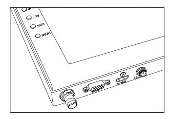
BNC – AV Composite Input VGA – Video Graphics Array DE15 Connection HDMI – High-Definition Multimedia Interface Input Connection Power Port – 12-24v Input
