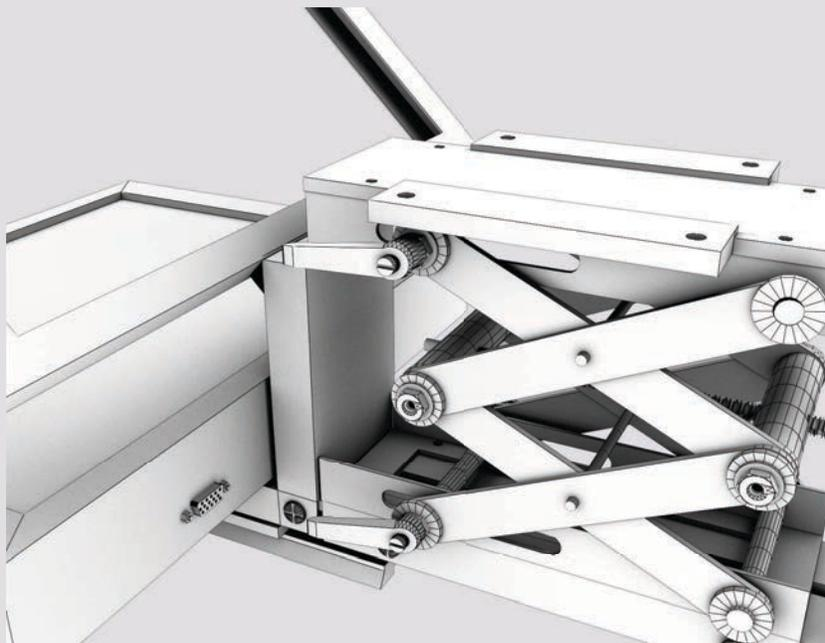
Attach the Quick Release Plate onto the Camera Lift with four 1/4-20 Mounting Screws.
