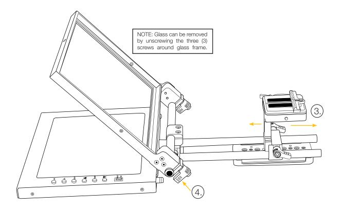
4. Tighten & Loosen thumb screw to adjust glass frame. Ideal angle is 45 Degrees.
