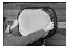
**Step 5:** Placing the soft box on the light and fitting it into place. The soft box will slip over the barn doors and slid around the edges of the light. The back flaps will fit around the light and the hook straps will attach to the loop patches on the side flaps.
