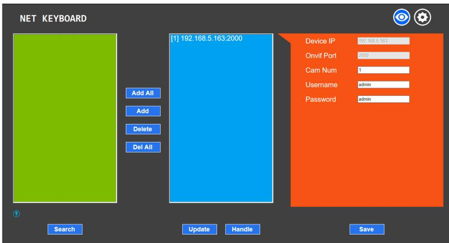
4. The home page consists of three segments: Search Device List (green); Added Device List (blue) or Manually Add (yellow); Device Details (orange).
