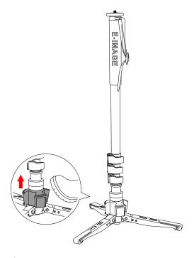
Step on the base part again to lock the monopod in upright.
