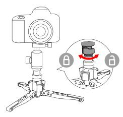
**5** Loose the bottom base of monopod to remove the monopod, the mini leg can be acted as a mini tripod, make low angle shooting.
