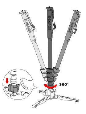
3 Step on the base part to release the monopod, it can swivel 360° and be tilted in any direction.
