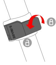
2 Open the flip locking to expand or collapse monopod tube.
