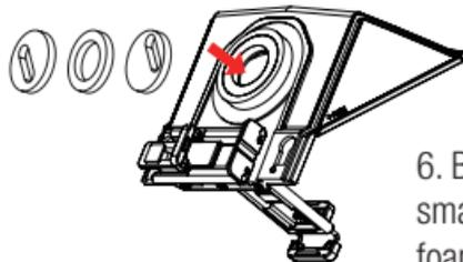
6. Based off the camera of your smartphone place one of the two foam rings into the adapter ring
