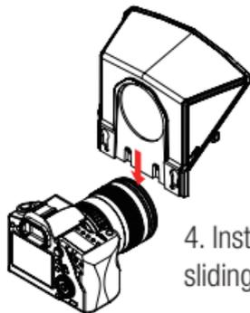
4. Install the teleprompter by sliding it over the ring adapter
