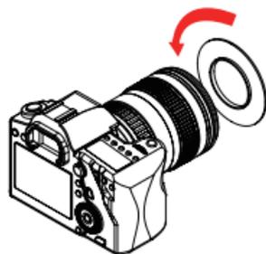
3. Install the lens adapter by screwing it to your lens. Make sure the adapter is screwed on completely.
