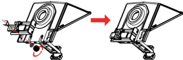
4. Unscrew the knob from the smartphone holder. Smartphone holder can be installed on either side depending on your preference. To record horizontal footages install smartphone holder vertically. To record vertical footages install smartphone holder horizontally.
